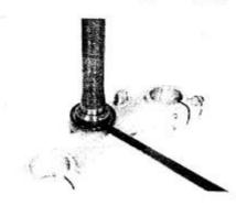
Push out the steering stem bearing races, upper and lower, with the special tools.
